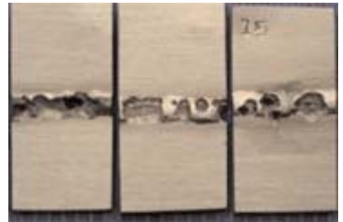
Soonv C-2000 alloy welded with matching filler metal.
