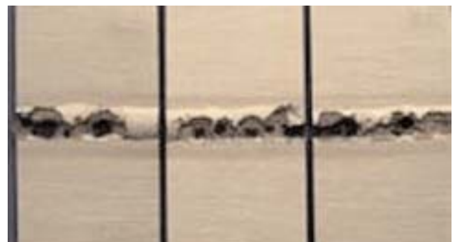
VDM alloy 59 welded with matching filler metal.
